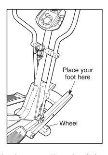
place one foot against the ramp and lower the elliptical crosstrainer. Due to the size and weight of the elliptical crosstrainer, use extreme caution while moving and lowering it.
